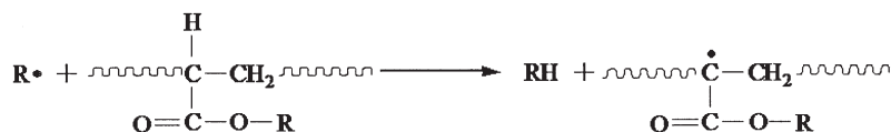
Scheme 2 Proposed branching site during the polymerization reaction. R represents the aliphatic portion of BA or MA. The long chains represent the polymer already formed.
